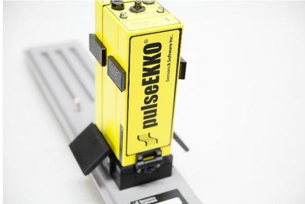
Connect the electronics boxes to the mounting block using the two plastic draw latch connectors.
