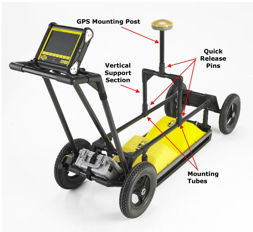
1. Fasten the U-shaped **Vertical Support Section** onto the **tubes** on the separation bars and secure it by inserting the 2 quick release pins.
