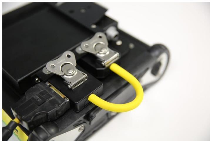
The female end of that cable can connect to the receptacle on the sensor head. When disconnecting the TR1000 cable from the TR1000 or the Adapter Cable, it is necessary to squeeze the connector release tabs on either side of the connector.
