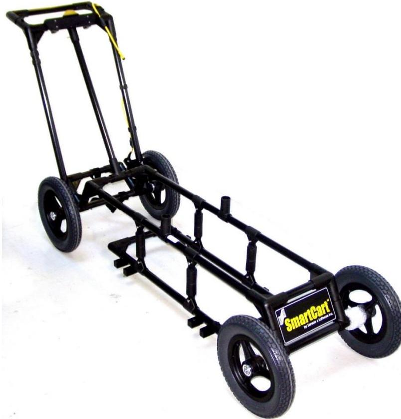
Each system has a unique set of separation bars to attach the transducers or low frequency antennas to the SmartCart and suspend them over the surface.
