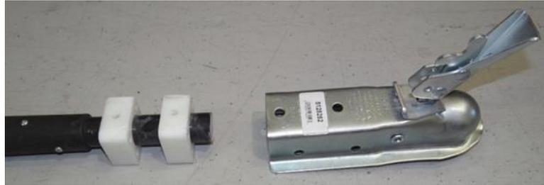
4. Place the Ball Hitch Receiver on top, lining up the holes.
