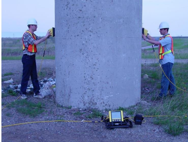
Figure 6-14: Transillumination survey on a column
