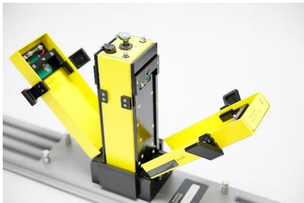
Place one 12-volt battery on each side of each of the electronics boxes. Make sure the positive (+) terminal faces inward toward the electronics.
