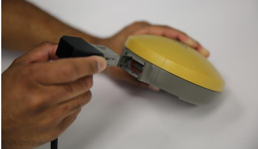
This single cable powers the GPS (if this option is turned on in the GPS menu) and receives data from it. Ensure that the DVL is powered down when connecting or disconnecting the GPS cable.
