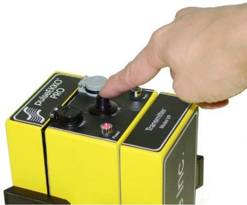
Figure 4-1: Turning on the Transmitter
