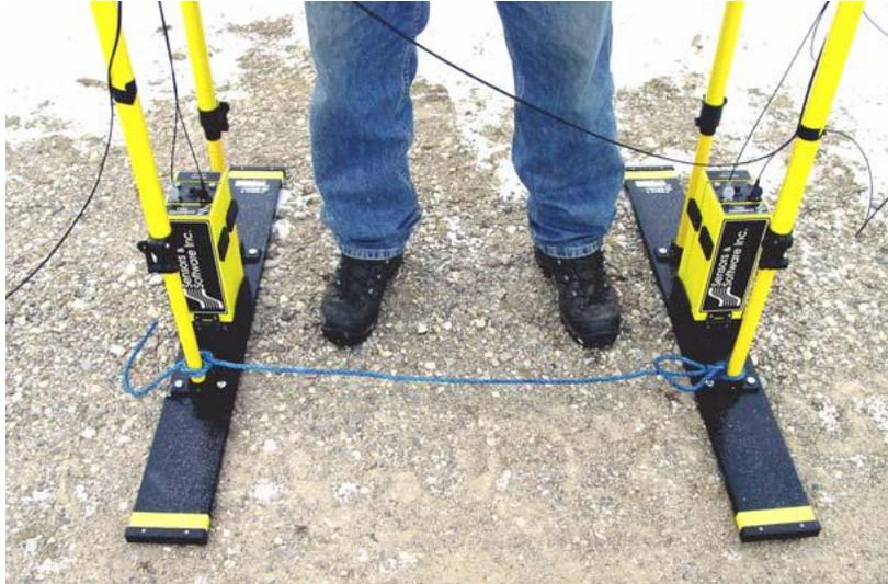
*Figure 11-2: Using string to keep antennas at fixed separation*
