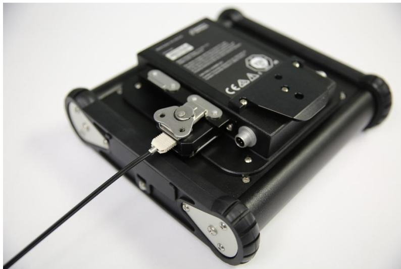
3. The next connection uses a special dual fibre optic cable, where both ends are identical.
