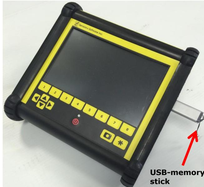
Figure 10-5: Insert a USB memory stick into the USB port on the DVL to export data.
