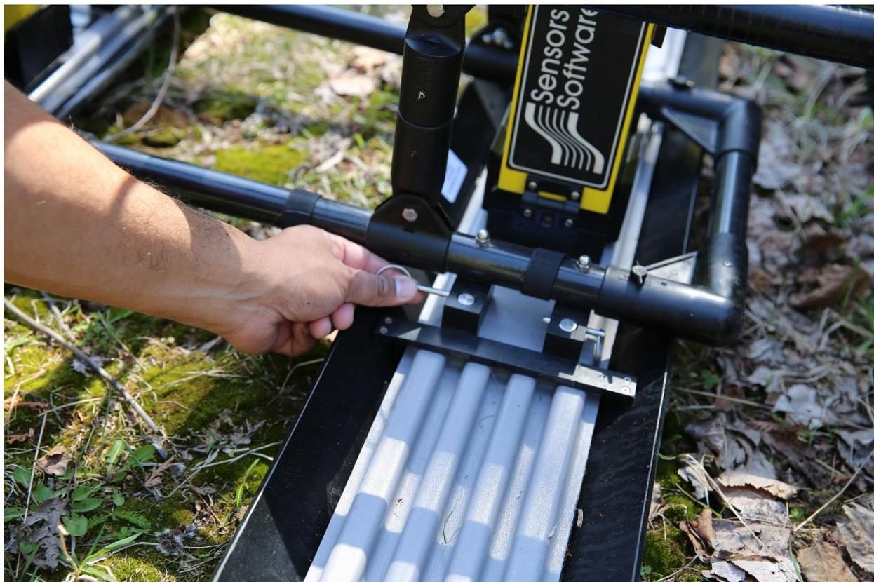
Attach the antennas to the SmartCart before attaching the transmitter and receiver (with batteries inside) to the antennas. To complete all cable connections, see section on [Connecting Fibre Optic Cables](#) (3.6.2). Once completed, the assembled SmartCart is shown below with 50
