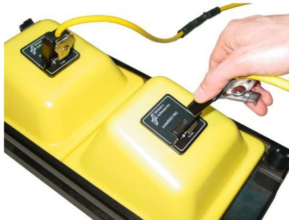
Connect the male end of the transducer cables from the transmitting and receiving transducers to the back of the DVL. The electronics recognize which device is connected to which receptacle. Secure the cable attachments with latches.
