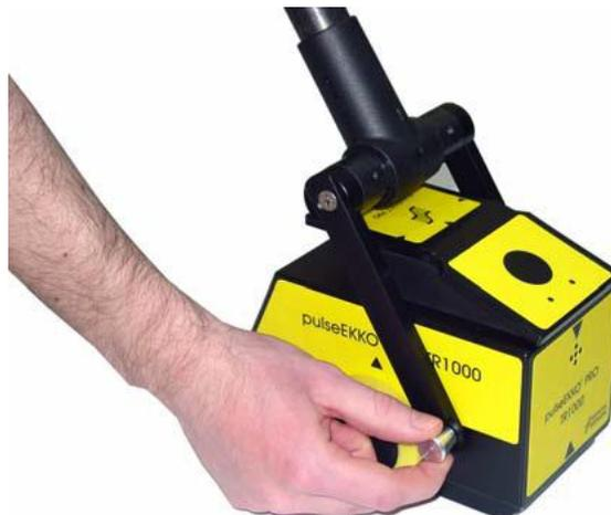
An assembled TR1000 with handle is shown below. When using the handle, a harness is typically used to support the DVL in front of the operator [Section 3.7.2](#).
