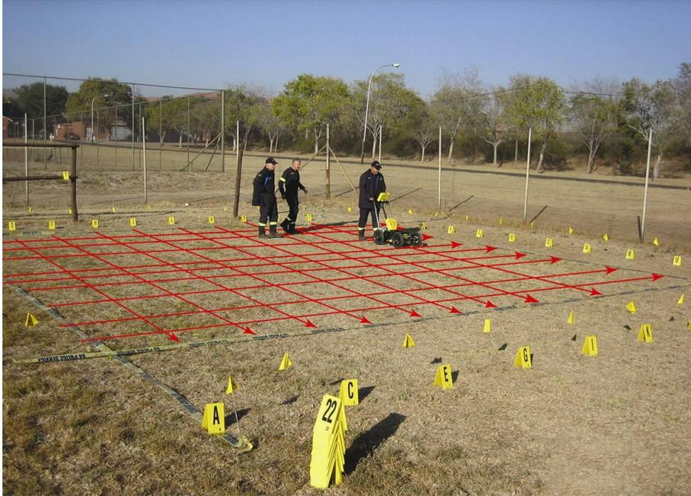
Figure 7-34: Example of a grid survey. The red lines are superimposed just to illustrate the concept.
