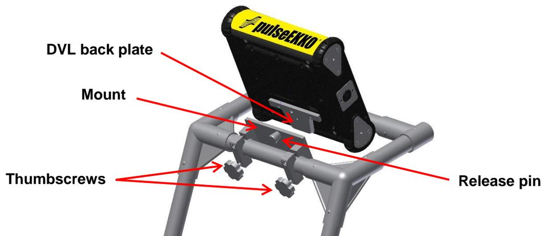
4. Rotate the DVL to adjust the view angle. If it is difficult to rotate, slightly loosen the thumbscrews on the bottom of the support shelf. Tighten to fix the viewing angle.
