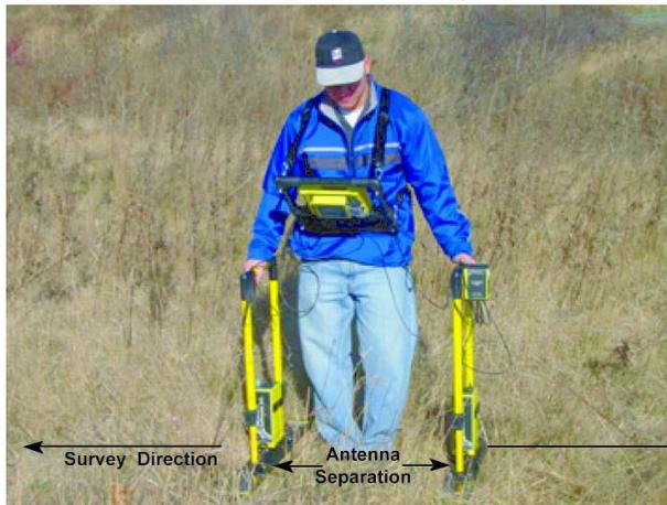
Figure 11-4: Antennas are held at the proper antenna separation for the selected frequency and perpendicular to the survey line direction.
