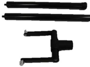
To connect the handle to the Sensor Head, slightly retract the 2 spring-loaded knobs on the end of the handle forks, align with the two holes at the back of the Sensor Head and release them to lock into position. Ensure that the cable remains below the handle to avoid stressing it.
