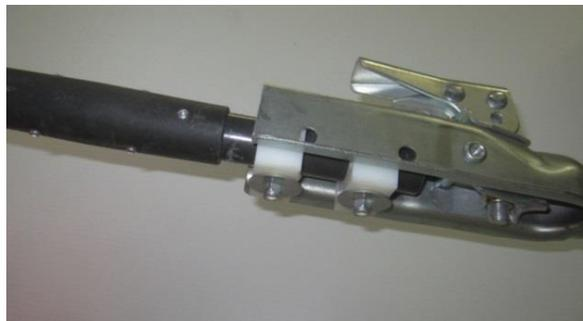
6. Tighten the bolts with a 7/16-inch wrench.
