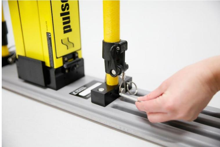
2. Adjust the handle height by loosening the two levers by hand.
