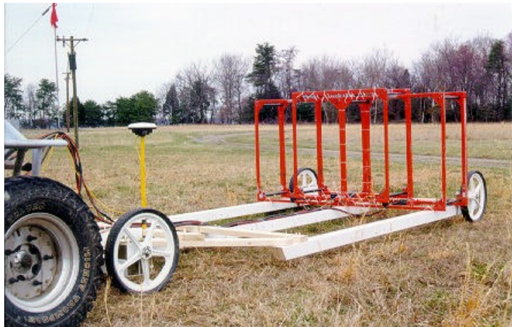
Figure 5 — The MTADS EM-61 array rotated 90°.
